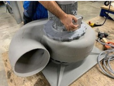
4. Turn the unit over and install the motor on the motor flange.
