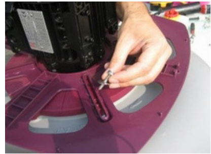
15-16-17. Fix the hat on the 4 remaining screw-in locations with screws and washers.
