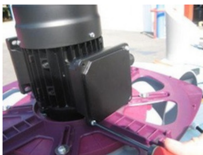
19. Screw terminal box cover back on.
