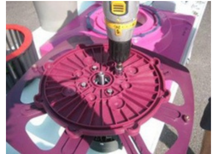
3. Secure the motor flange with the 4 screws.
