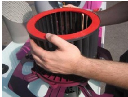
5. Position the impeller on the shaft.
