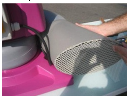
225. Place the diffuser on the fan housing outlet and secure with 1 screw.
