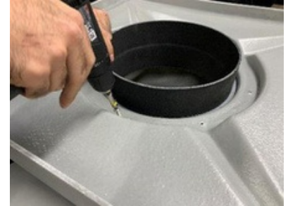
3. Screw stub to inlet flange.
