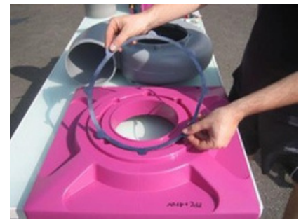
9. Place the O-ring on the stub.
