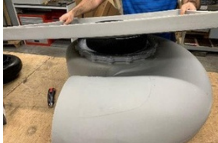
2. Install stump on suction flange.
