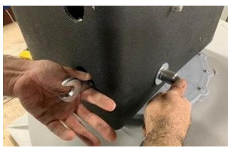
Use the holes on the side of the motor cap to access the bolts.
