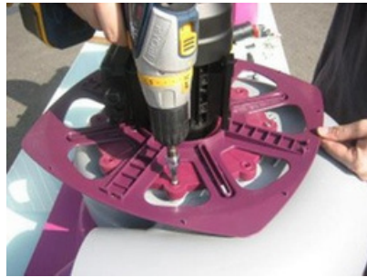
14. First screw in 4 screws at the 4 cardinal points to secure the flange to the fan housing.
