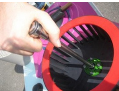
7. Screw the hub onto the motor shaft using screw + washer.
