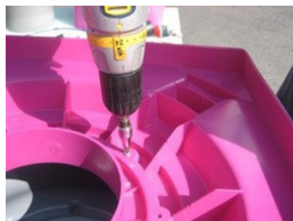
11. Screw the stump to the fan housing.
