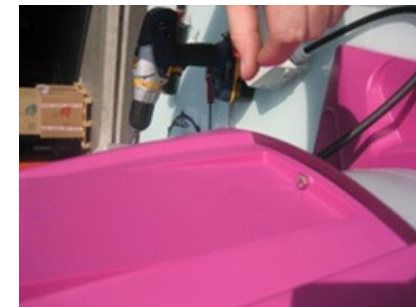
20-21. Position the motor cap and secure with screws.
