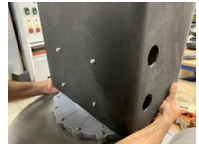
6. Place the motor cap on motor and match the holes and screws.
