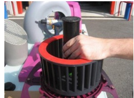
6. Use a mallet to press the impeller.
