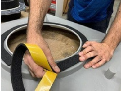
1. Tape the flat gasket to the stump.
