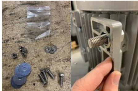
5. Insert the 4 screws on the motor and secure with vistop washer.
